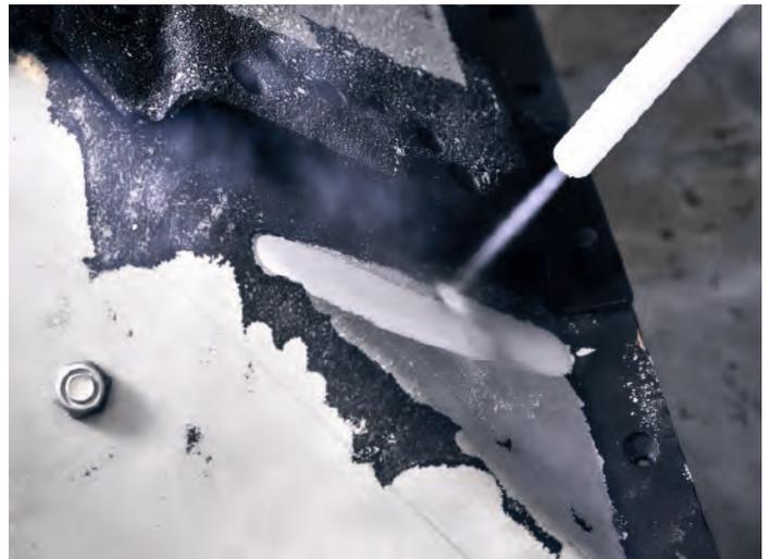
The hard way or the soft way? With the PCS 60, Cold Jet has for the first time developed a dry ice blasting system that allows users to choose between 28 particle sizes.
